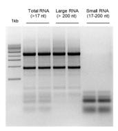
RNA Clean & Concentrator™ allows for clean-up of total RNA (> 17 nt), large RNAs (> 200 nt), and/or small RNAs (17-200 nt).
